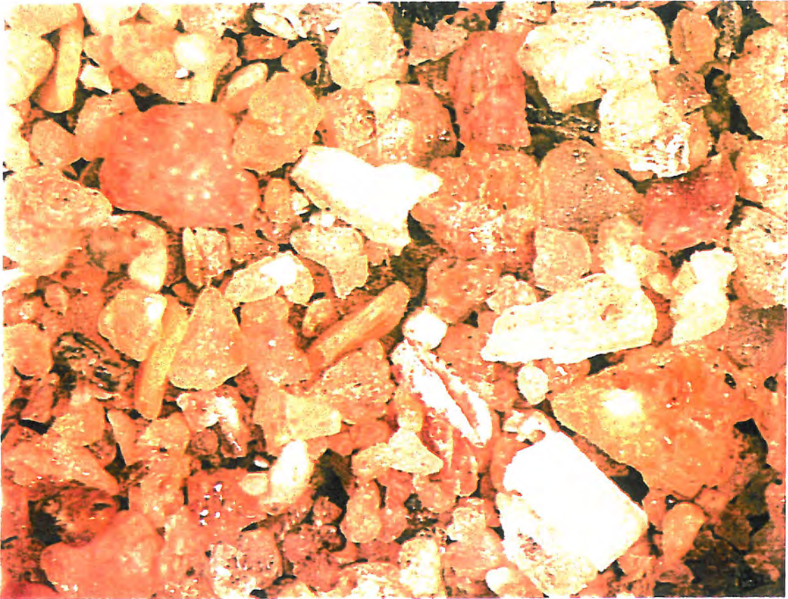
Area 1 core sample C1-9. Well sorted, medium-grained, subangular to subrounded clean sand. Magnification (X16) Field of view 4.6 mm by 3.6 mm.
