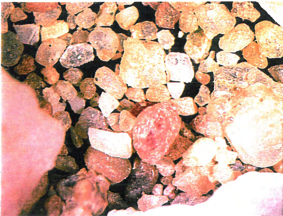
Area 1 core sample C3-3. Moderately well sorted, medium-grained, subangular to well rounded. Note coatings of mud or calcium carbonate on some of the grains. Magnification (X16) Field of view 4.6 mm by 3.6 mm.
