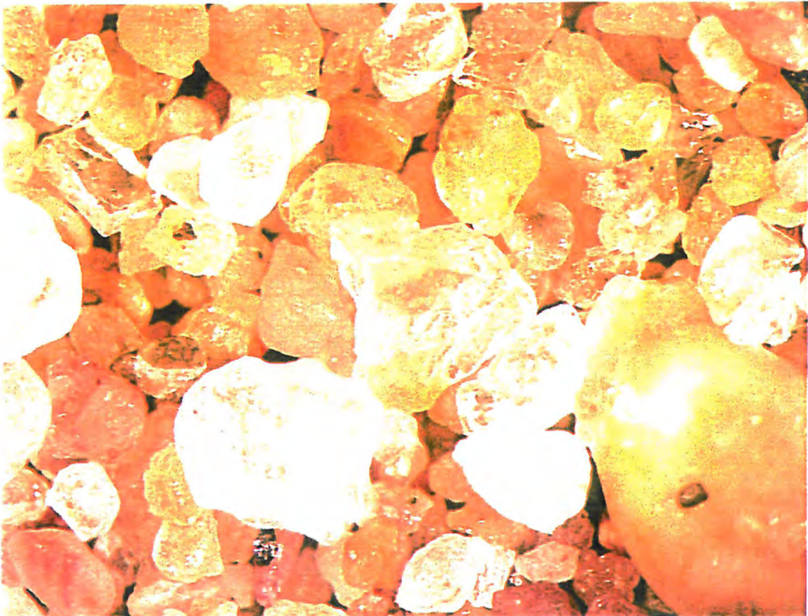
Area 1 grab sample G23. Well sorted, medium-grained, subangular to well rounded clean sand. Magnification (X16) Field of view 4.6 mm by 3.6 mm.
